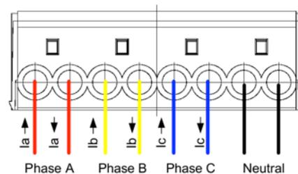
In the case of direct three-phase connection (up to 100 A), you must connect the 3 phases and the neutral respectively to the following terminals:
