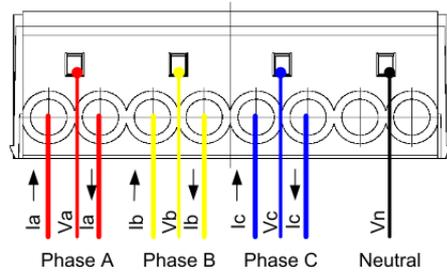
For an installation > 70 kWc, you must use Current Transformers (CTs) to measure the current. The transformation ratio must be specified with the order. You must then connect each CT on the Phase A, B and C inputs and finally supply the meter with power by connecting the phases and neutral on the Va, Vb, Vc and Vn inputs.
