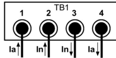
Connect the inverter's output to the meter's input (TB1). Phase must be connected to terminal 1, neutral to 2. Then connect the Mk7C meter's output to the power grid. Terminal 3 is neutral, 4 is phase.
